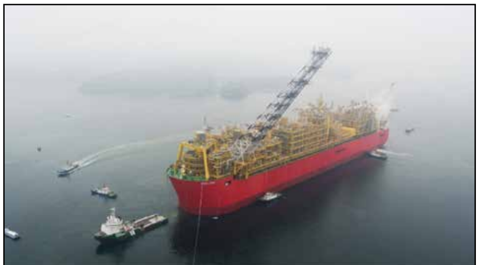
Shell’s Prelude floating liquified natural gas (LNG) processing facility is the world’s largest floating object. Photo: Shell Australia
