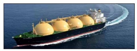
LNG ships like this one wil sail into Eastern Australian terminals and discharge gas at -161°C – usually to another vessel, a floating storage annd regasification unit (FRSU). Seawater is used to warm and regasify the liquid. Photo: APLNG
