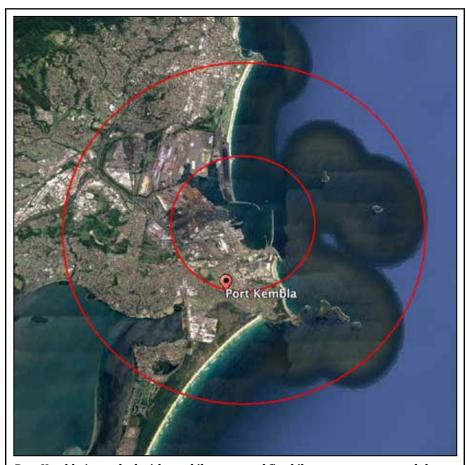
Port Kembla is marked with two kilometre and five kilometre zones around the harbour. If an accident occured at the proposed LNG import and regasification terminal, there is the risk of a boiling liquid expanding vapour explosion (BLEVE). Death and injury are likely within two kilometres, while debris could be ejected for up to five kilometres. (See FFB1.25 for more information on BLEVE dangers.) Picture: Google Earth
