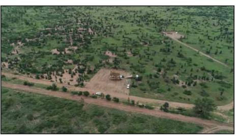
Disturbance site - Pad 2. The image was taken between April - May 2019 showing a cleared vegetation site. The image also displays site activities including a drilling rig, driller sumps, and vegetation storage. Photo: Coast and Country
