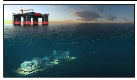
A seabed compressor will pump gas to the Gorgon LNG plant. Photo: Chevron
