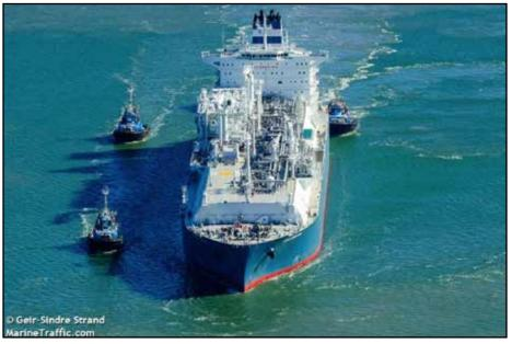
Hoegh Esperanza, the floating gas import terminal which AGL now plans to use at Crib Point, instead of the Hoegh Giant. It is understood the Esperanza uses gas, instead of seawater, to re-gasify LNG. It will create more carbon emissions, but won't be releasing tonnes of chilled, chlorinated water into the surrounding Ramsar-listed wetlands. Photo: Marinetraffic.com
